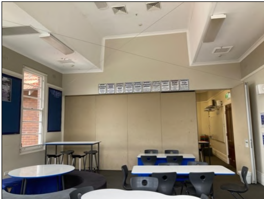
Figure 37: Classroom on the first-floor showing a contemporary operable divider with another classroom beyond. These dividers will be removed.
